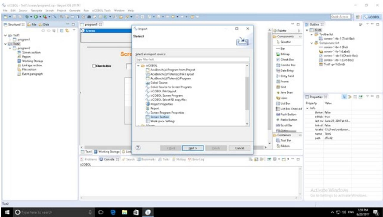
in the Import Screen Section window, expand the target project and select the target program, then browse to the location where you saved the .isl file and select it, then click finish.
